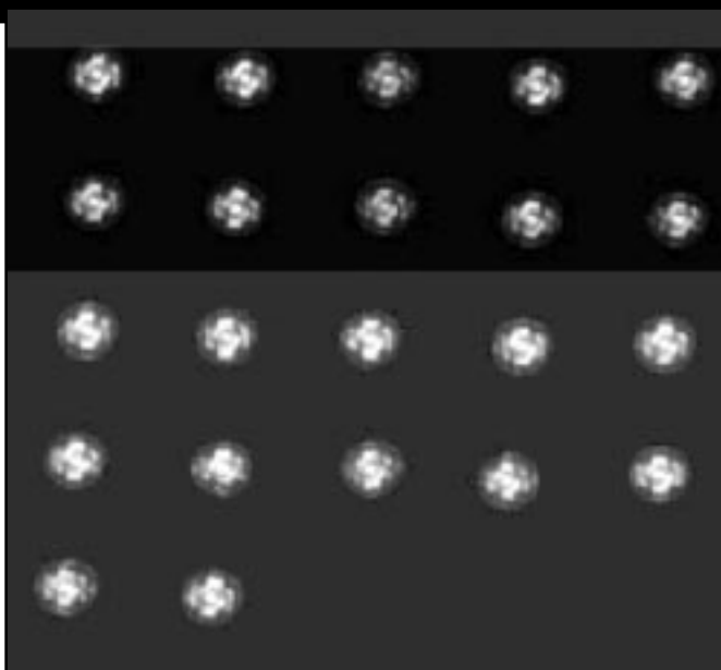
Figure 4b. Picture shows the scanning electron analysis result of Micro X plastic units that were built by using improved design. No delamination was observed after.
