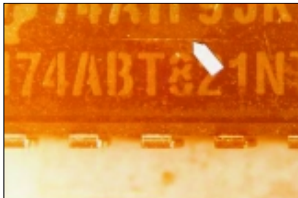
Photograph 1. A hairline crack in the plastic encapsulation.
