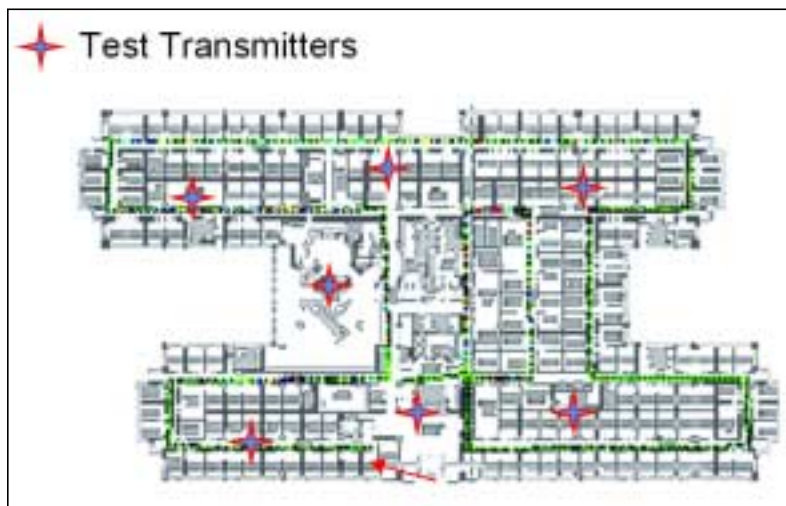
Figure 1. An example of a typical test transmitter setup for a site.
