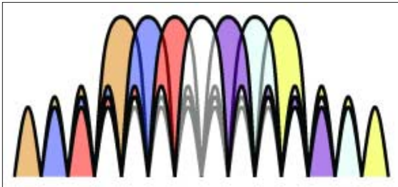
A typical set of OFDM carriers.
