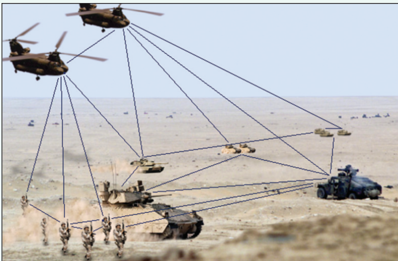
Ad hoc peer-to-peer wireless networking, or mobile mesh networking, can link battlefield forces without fixed infrastructure.
