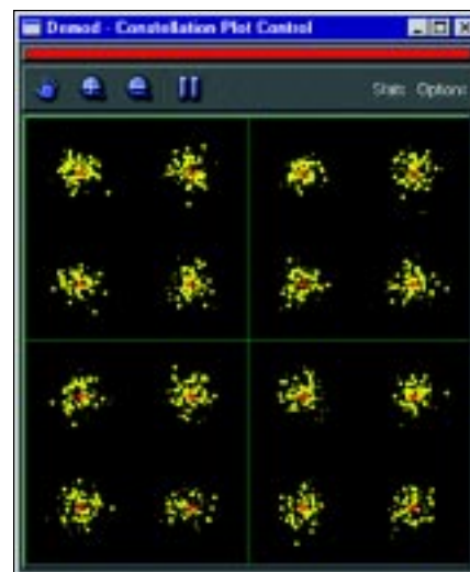
Figure 6. Passband amplitude and phase variation effects on 16QAM signal (without equalization).
