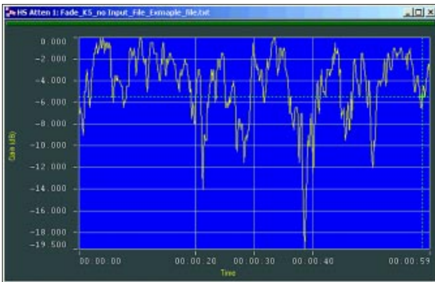
Figure 8. Received power over 60 seconds with a Ricean simulator module.
