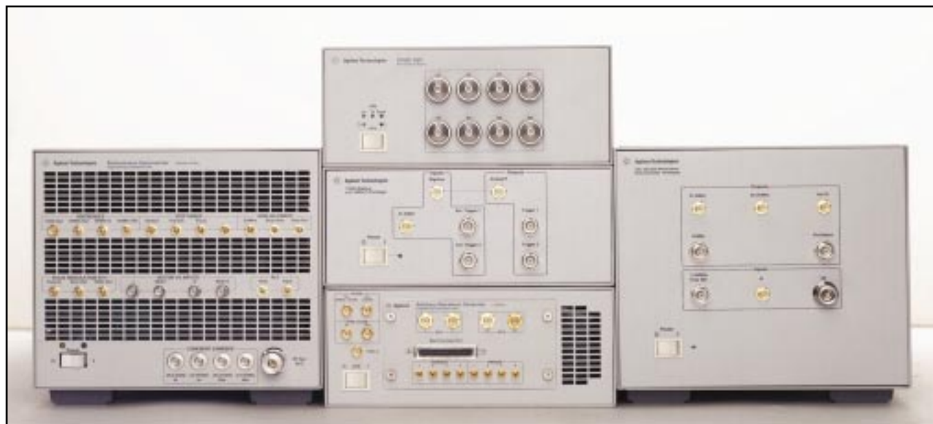
Figure 2. A prototype synthetic instrument system developed by Agilent Technologies incorporates various SI modules that emulate the stimulus and measurements functions of conventional test equipment.
