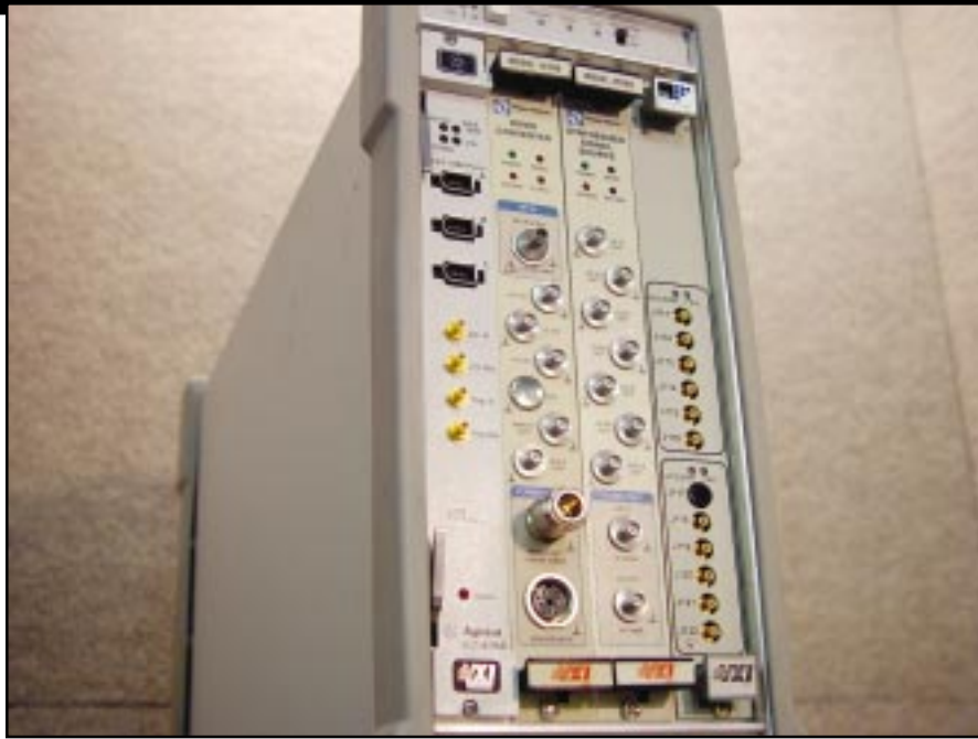
Figure 3. This SI combination of a Phase Matrix downconverter and local oscillator provides a modular microwave front-end based on the VXI bus architecture for ATE systems.
