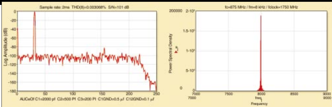
Figure 4. Performance of delta-sigma A/D converters using (a) CMOS technology and (b) GaAs MESFET technology.
