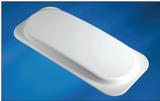
Figure 2. The M/A-COM MAANAT0123 antenna for the U.S. market (902 MHz to 928 MHz operation) features 6.5 dBi typical, VSWR of 1.4:1 typical and 10 K \Omega sensing circuit resistor. It measures just 19.6 inches x 8.8 inches x 1.6 inches.
