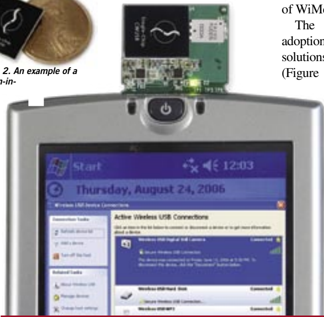
Figure 3. This add-on card from Staccato Communications, the SDIO card (SC3226R SDIO for native Certified Wireless USB), uses a single-chip CMOS SiP packaged solution.
