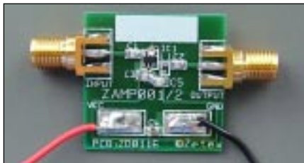
Figure 1. Amplifier test circuit board.
