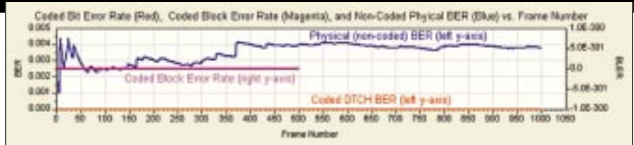
Figure 7. 1000-frame WCDMA BER measurement with simulated fading using a signal source streaming data file created with an EDA simulation.
