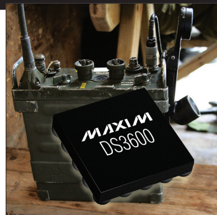
Figure 3. The CSBGA package of the DS36XX family provides a layer of passive protection by limiting access to I/O signals when the device is installed on a circuit board.
